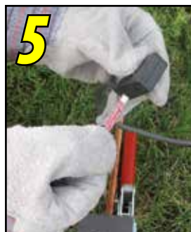
5 Insert the EZ Lite® Ignitor in the connector.
