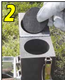
2 Place filter pad into lid.
