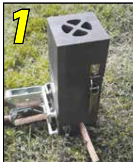
1 Position cleaned conductors in mold.
