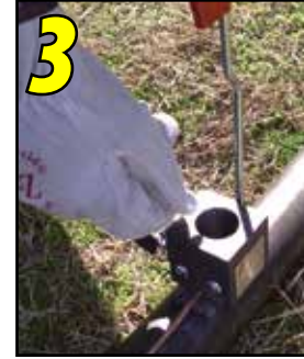
3 Place metal disc in bottom of mold.
